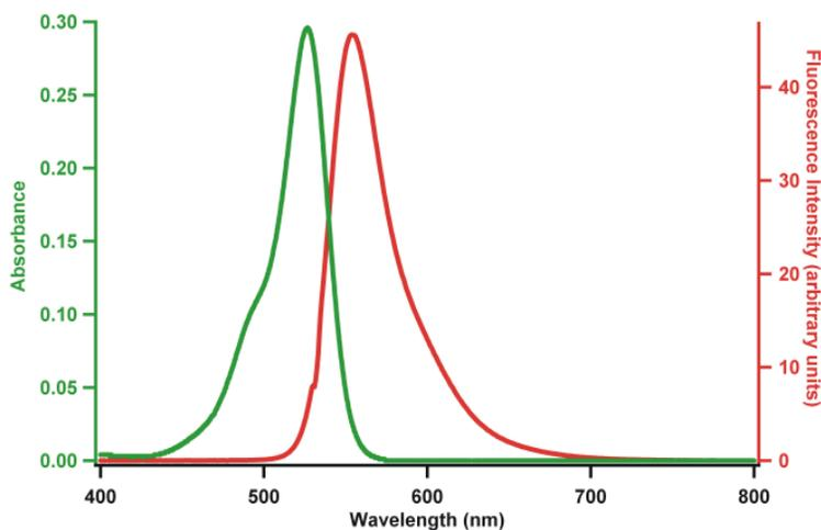
FIG. 3. Absorption (green) and emission (red) curves of Rhodamine 6G dye.
