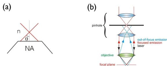
FIG. 2. a. The numerical aperture  $NA$  of a lens is given by  $NA = n \sin \theta$  where  $\theta$  is defined as illustrated here. b. Light emitted from the focal plane can be selectively detected by placing a pinhole in the image plane of the focus. As illustrated here, out-of-focus emission is not focussed by the first lens onto the aperture of the pinhole and thus is not detected further downstream. (Figure courtesy of Marcia Levitus, Arizona State University.)
