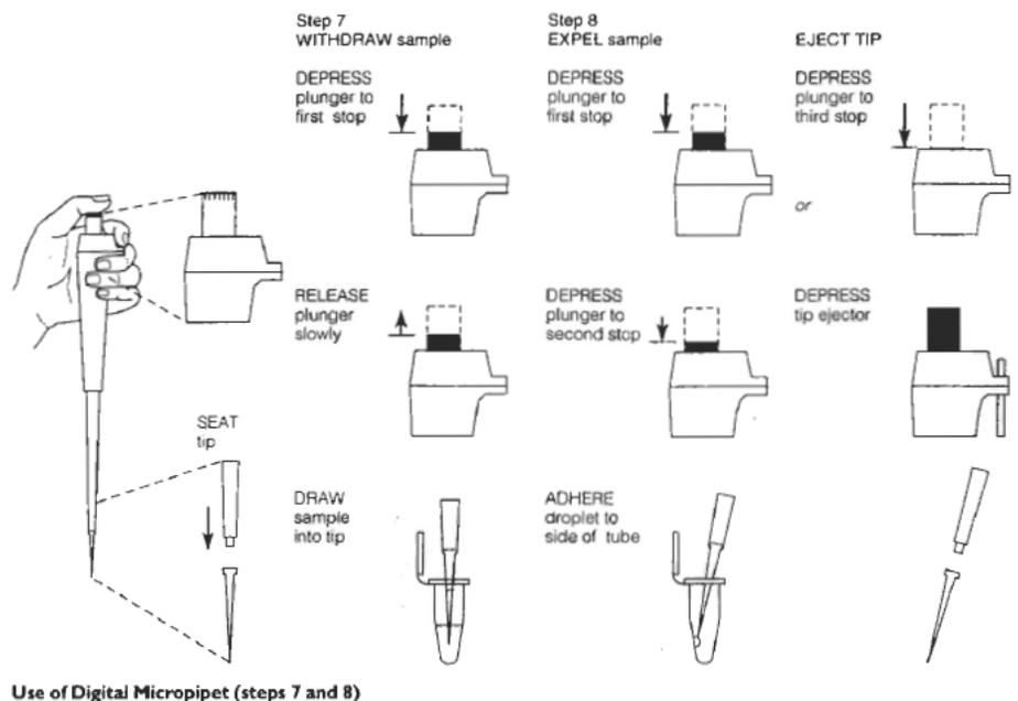
FIG. 1. Figure showing proper use of micropipette. (From *Laboratory DNA Science*, by Bloom, Freyer and Micklos, The Benjamin/Cummings Publishing Company, Inc., 1996, p. 8.)
