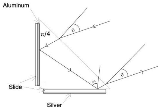
Fig 4. Diagram of light propagation path through the prism.
