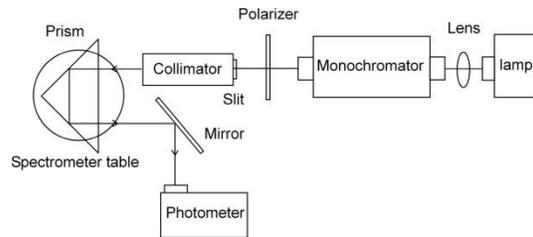
Fig. 2. Schematics of experimental setup for surface plasmon measurement
