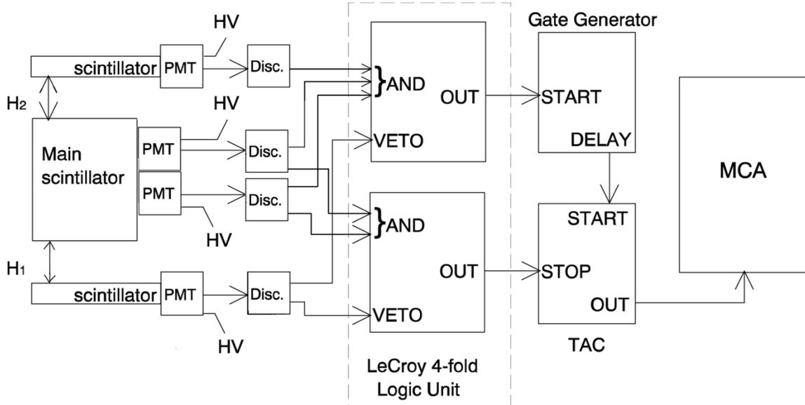
Figure 3. Alternative setup with coincidence and anticoincidence requirements.
