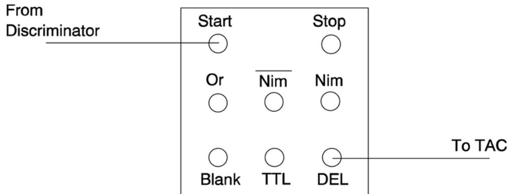
Figure 2. LeCroy Gate Generator used to delay START pulse.
