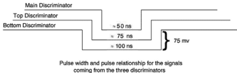
Figure 4. Timing information for the coincidence/anti-coincidence setup.
