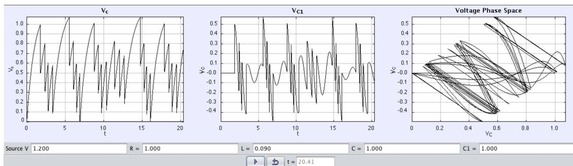
Fig. 4 A simulated run of the autonomous relaxation oscillator. The firing of the neon lamp (labeled Ne in Fig. 2) is apparent in the sharp corner points in all three plots.
