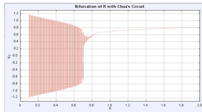
Fig. 5 The long-term voltage values in  $C$  in Chua's circuit, plotted against  $R$ . Low values lead to periodic oscillation, and high values lead to a flat, stable voltage, but values between 0.682 and 0.703 produce chaos.
