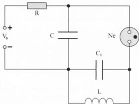
Fig. 2 An autonomous relaxation oscillator
