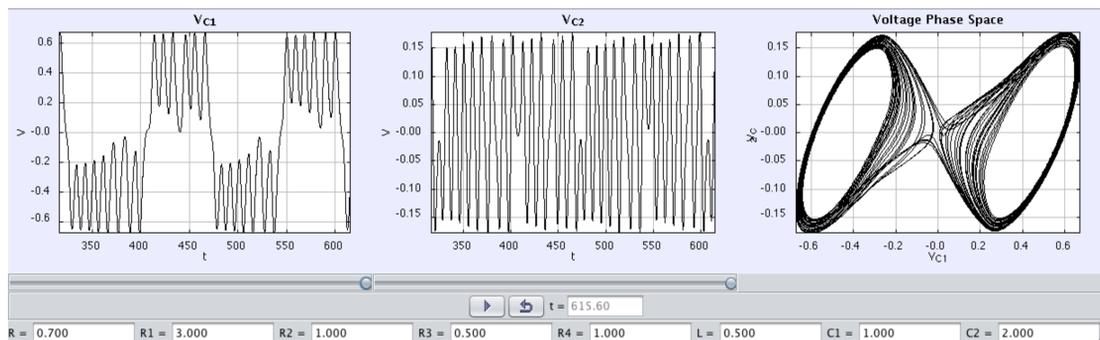
Fig. 3 A simulated run of Chua's circuit with the listed initial conditions
