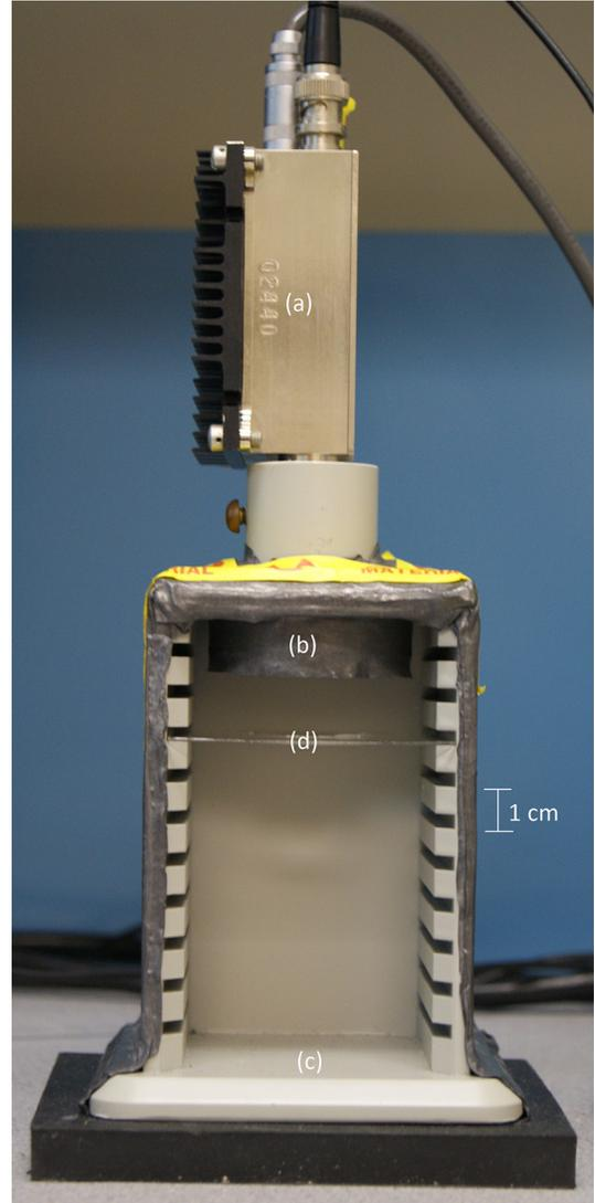
Fig. 1. The experimental setup including the detector (a), shielded source array (b), lead lined plastic stand (c), and plastic sample tray (d).
