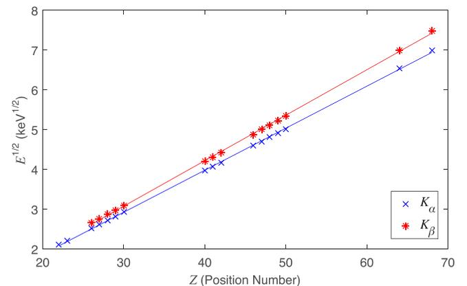
Fig. 5. Plot of the square root of  $K_\alpha$  and  $K_\beta$  X-ray energies versus  $Z$  along with a best fit line for each transition.
