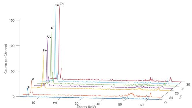
Fig. 3. Overlay of first row transition metals spectra.
