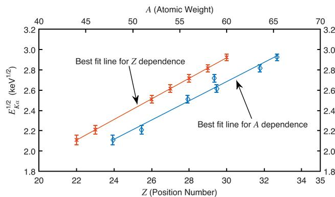
Fig. 4. Plot of the square root of the characteristic  $K_\alpha$  X-ray energies versus  $Z$  and  $A$ . The energies of the  $K_\alpha$  X-rays correlate much better with  $Z$  than  $A$ , confirming Moseley's conclusion.
