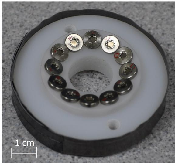
Fig. 2. The source array used to excite the metal foil samples. The exterior of the array is covered in lead foil to shield the sources.
