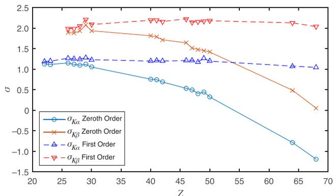
Fig. 6. Zeroth- and first-order screening constants for all samples. Applying a first-order correction to Moseley’s law causes the screening constant to be more “constant,” however, there is still some residual curvature towards high  $Z$  elements.
