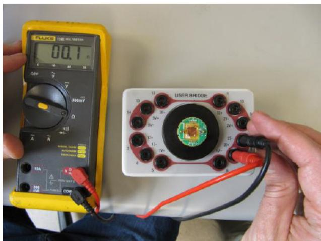
Figure 9. Testing connections on the VersaLab puck via the sample test holder accessory.
