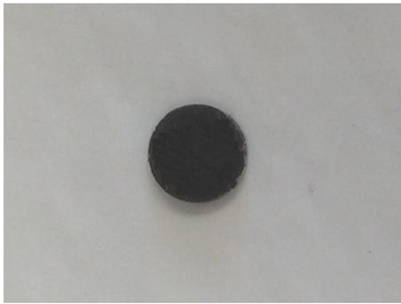
Figure 1. Completed YBCO pellet.
