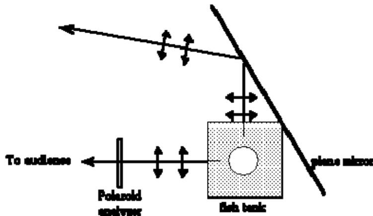
Cuvette and mirror, looking into the beam. (Fig 2)
