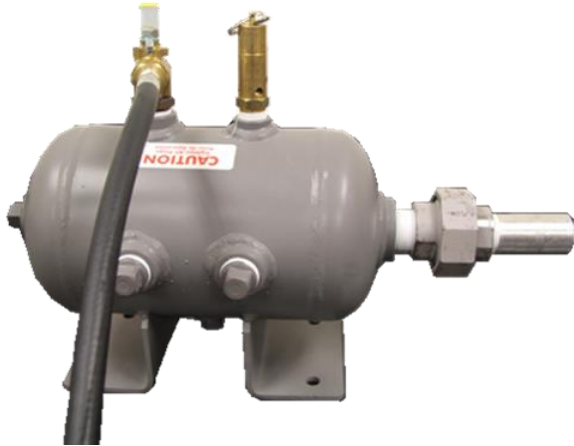
FIGURE 1. Nozzle flow apparatus: Pressure tank and nozzle. The 1-gallon ASME-code horizontal compressed air tank is available through McMaster.com.
