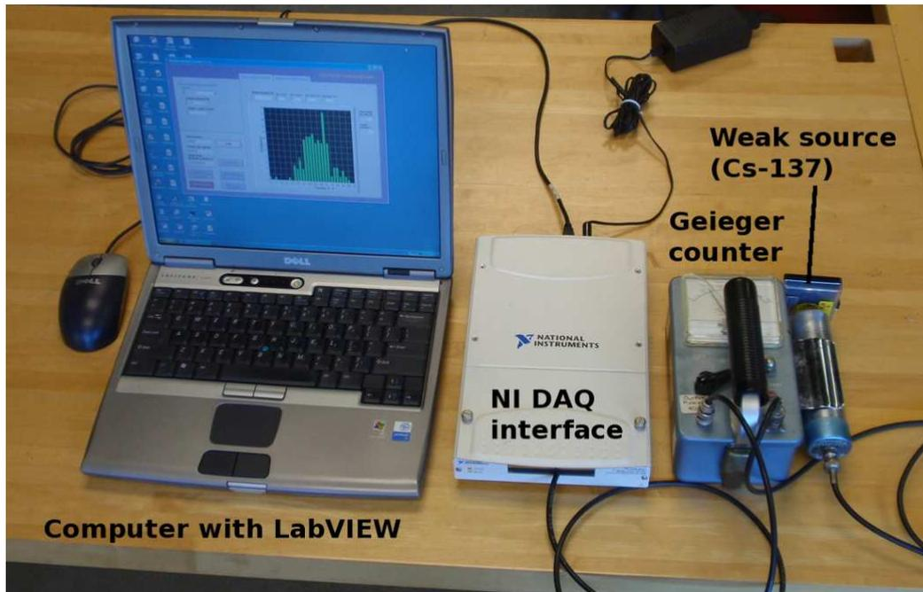
Figure 5: Minimal setup needed to count random pulses from a Geiger counter. The survey meter has a TTL level output that feeds directly into the counter gate on the DAQ interface. A computer with LabVIEW collects the data and the LabVIEW program allows analysis in a variety of ways. When used with the cosmic rays setup the output of the LeCroy 222 gate generator replaces the Geiger counter.
