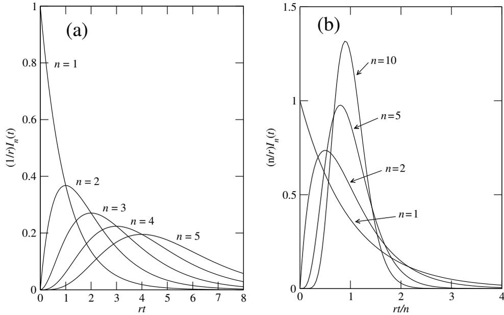
Figure 6: The  $n$ -pulse interval density functions, after Knoll [2, p. 98]. (a)  $(1/r)I_n(t)$  for  $n$  from 1 to 5. Notice that the functions peak at  $rt = n - 1$ . (b)  $(1/r)I_n(t)$  scaled by the transformations  $t \rightarrow t/n$  and  $(1/r)I_n(t) \rightarrow (n/r)I_n(t)$  to show that as  $n$  increases, the function becomes more sharply peaked around the mean value  $\tau_n = n/r$ .
