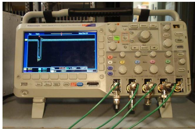
Figure 4: Oscilloscope showing simultaneous fast NIM pulses, indicating the passage of a cosmic ray muon through all paddles.
