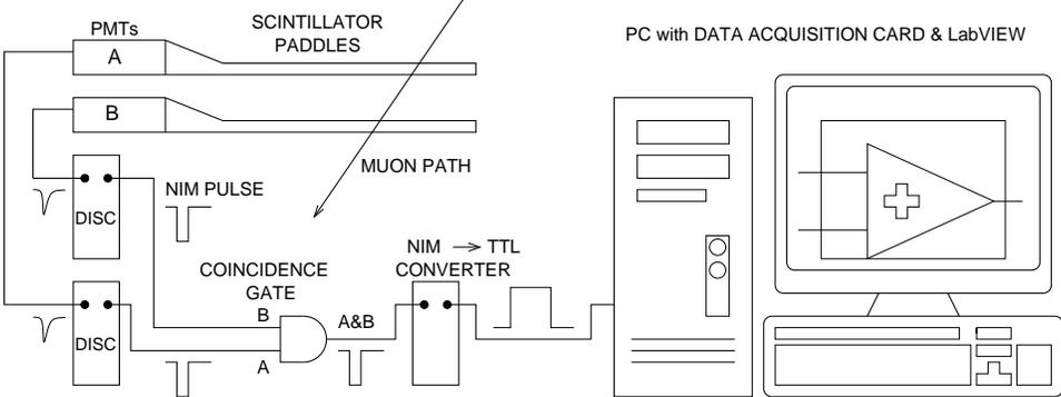
Figure 1: Schematic of the muon telescope apparatus. Although there are only two scintillator paddles shown in the figure, the actual setup uses between three and four paddles. The AND gate is a 4-fold NIM logic unit. Data are collected with the LabVIEW Interval Counter software.
