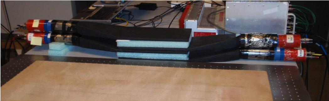
Figure 2: Stack of scintillator paddles used to count cosmic rays. Scintillator material is 12"  $\times$  6"  $\times$  1cm. It is glued to a Lucite light pipe, which is wrapped in aluminum foil and heavy black paper. Each assembly is attached to a 10 stage PMT (Electron Tubes 9266KB). The high-voltage bias is between 800-1100 volts. High energy muons pass through all paddles, creating a set of coincident pulses.
