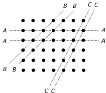
Here the planes AA, BB, and CC represent the various orientations the powder crystal could have. In a powder sample, each plain is equally likely to be in line with the X-ray beam. However some plains in various crystals will be less likely to forward scatter than others. Each powder sample has its own unique diffraction pattern depending on its plane spacing and lattice structure.
