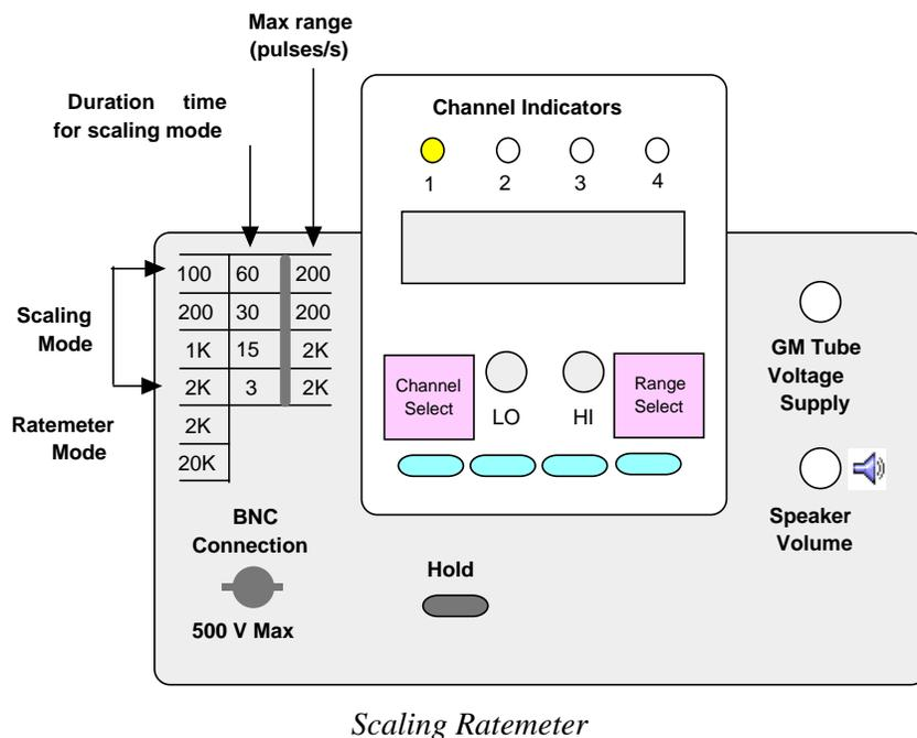
**Ratemeter Mode:** In this mode, the count rate (pulses/s) is displayed on channel 1. The counts can be displayed in two ranges of 2 k and 20 k pulses per second depending on the switch selection.
