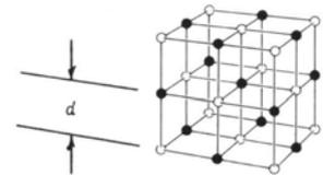
Using the provided values for sodium chloride, estimate the spacing distance  $d$  for this crystal. How does this value compare to your experimental measurement?
