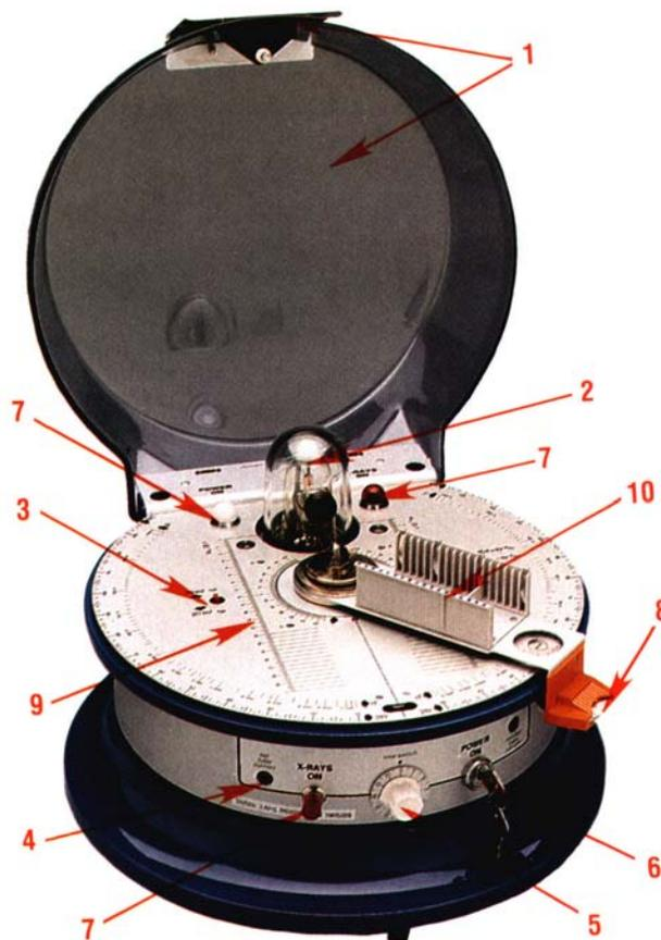
7. Warning lights which illuminate to signal when the power is on (white light) and when x-rays have been turned on (red light).
